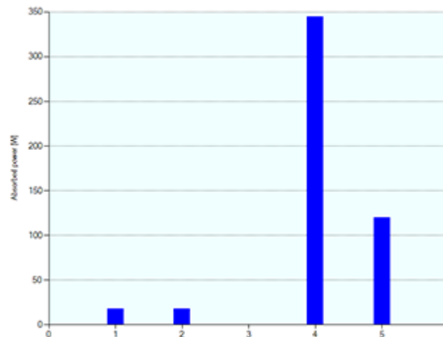
Figure 6.10: In position 1 and 2 we have the Athena 311 FCC. In position 4 is indicated the power used by G1000, and in position number 5 is indicated the dedicated HUD from
