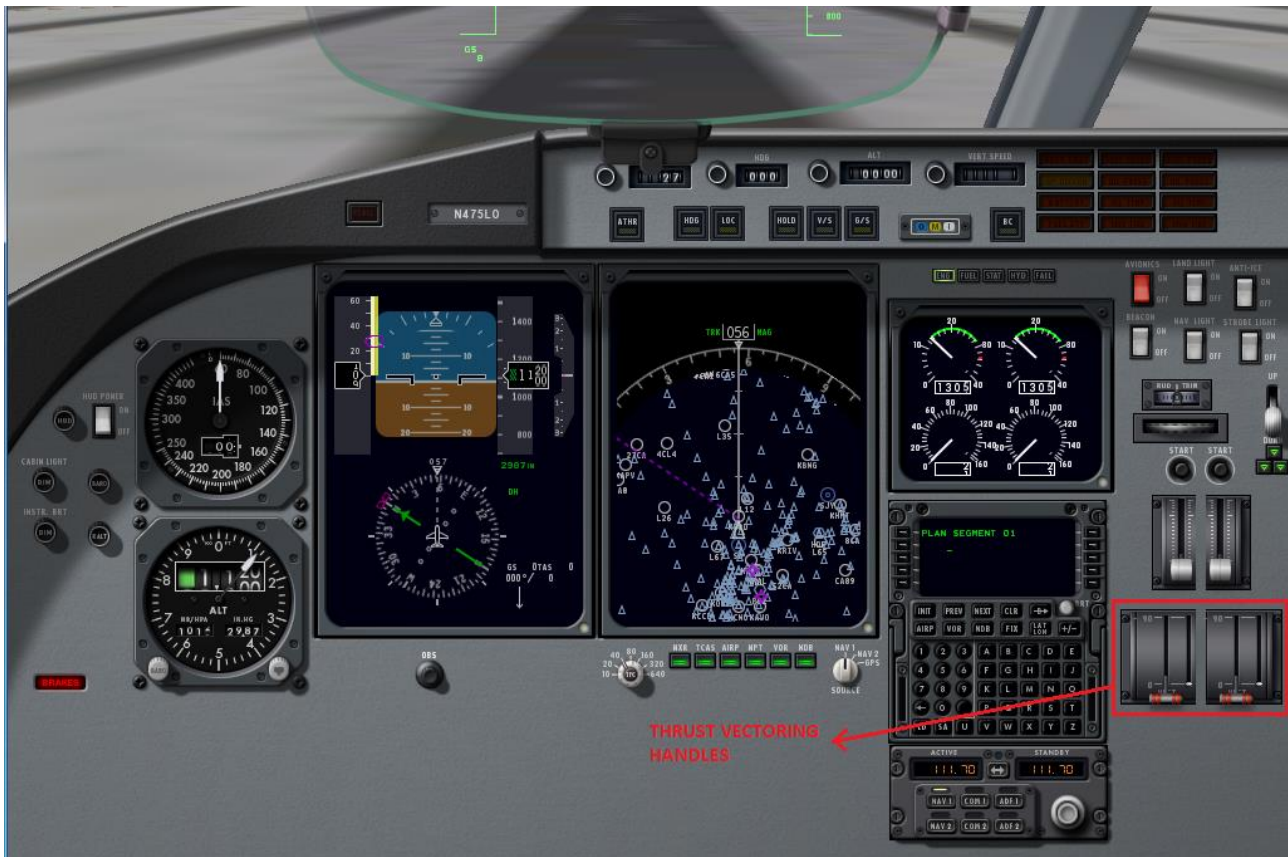
Figure 14.14.10: Panel details in X-Plane with indication of thrust vectoring handles
