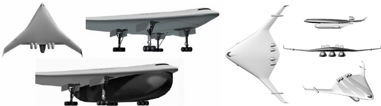
Figure 12: CAT large flying wings with 2 versions of detachable pods (Snead, 2005)
