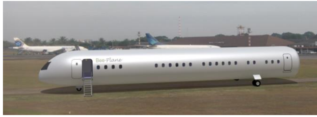
Figure 24: Bee-Plane detachable fuselage on an airport (ESTACA, 2013)
