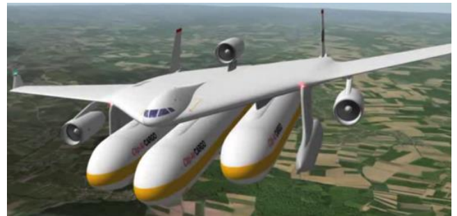
Figure 11: Clip-Air flying wings with detachable fuselages (EPFL, 2012)
