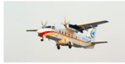
Y-12F The Y-12F is the latest dev wing, unpressurized cabin, retractable landing gear, single ver.....
