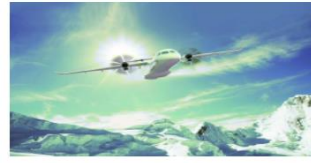
MA700 The MA700 is a new generation of turboprop regional aircraft with a high-wing, T-shape tail, wing-hanged twin engines, composite propellers and tricycle landing gear configuration. It is a two-pilot aircraft with a standard cabin layout of 78 seats..... learn more
