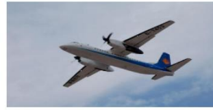
MA60 The MA60 is a two-pilot aircraft carrying 52-56 passengers. The main avionics are from world-famous suppliers and it is equipped with two PW-127J turboprop engines of Pratt & Whitney Canada and 247F-3 propellers of Hamilton Sundstrand of US. learn more
